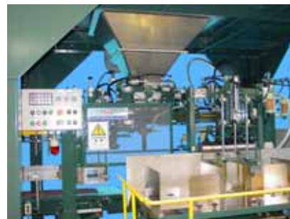
Operating panel, bag magazine and filling device
