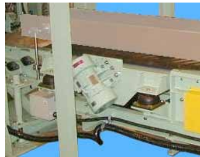
Air ridding device by vibration on conveyor
